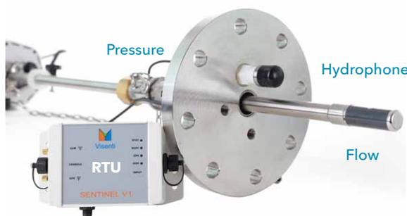
The sensing devices transmit continuous information about potential leaks in the pipe network to a data management and analytics engine. The LeakView™ system identifies the pressure transients, acoustic noise and/or flow anomalies related to such breaks and localizes them to the faulty pipe with high likelihood. This detection process is automated and provides information on the severity of leaks to help the repair crews prioritise their response.
